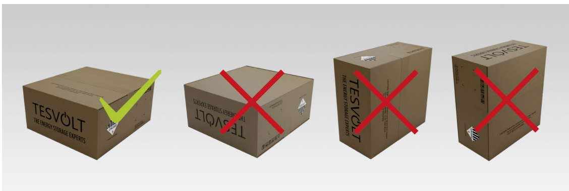
Figure 3.1 Permissible and impermissible storage positions of a packaged battery module
