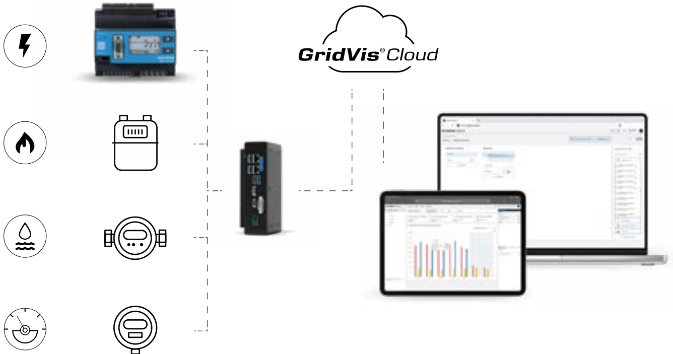
Fig.: GridVis® Cloud system architecture
