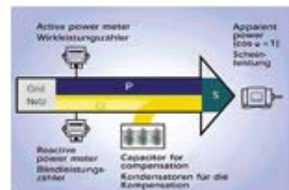
Fig.: Principle of power factor correction
