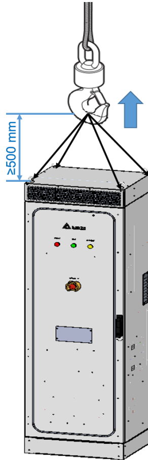
Figure 12. Eye Bolts Lifting
