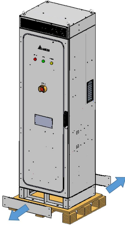
Figure 17. Removing Front/Rear Base Covers
