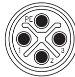
3+PE-pos. S-coded for power supply
